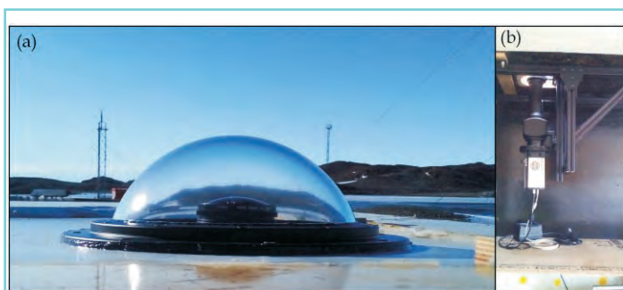
Figure 5 Left Panel: Fisheye lens of GRAAS covered by Optical grade BK7 Glass dome. Right Panel: Coupled Optical Assembly and CCD detector of GRAAS.
