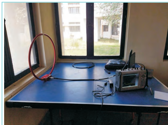
Figure 33 Loop Antenna Setup used for Noise Survey by SAMEER team at KSKGRL, Prayagraj, UP
