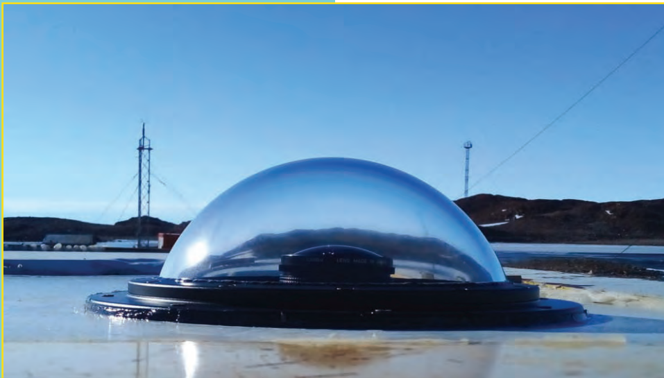
"Hemispheric observing dome of the Grism-based Spectrograph for Airglow & Auroral Studies installed at Maitri, Antarctica.
