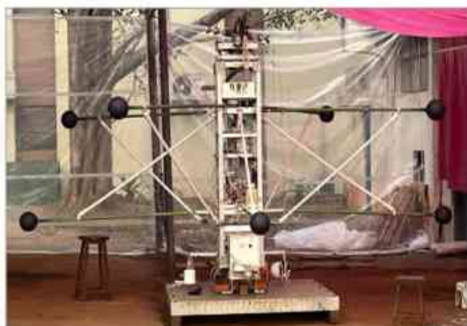
Figure 13 Photograph of BEENS payload depicting the spherical probe sensors attached to 2 m long booms.
