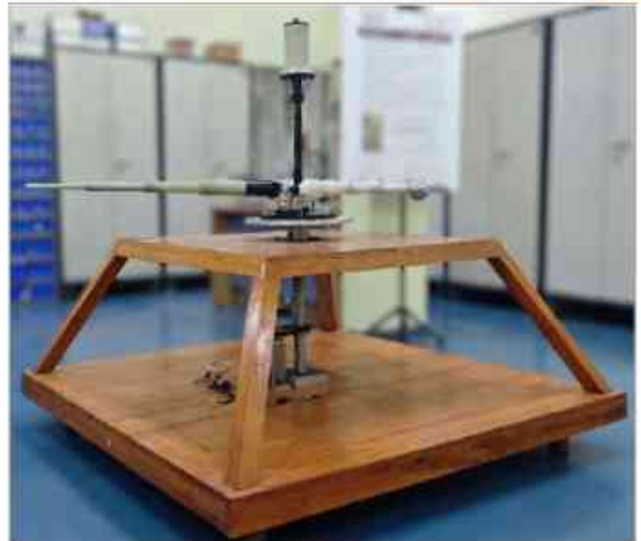
Figure 5 Spinning stability test on Rotating platform
